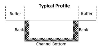
**Note:** This profile represents a typical Gabion ditch. Depth and buffer area varies.
