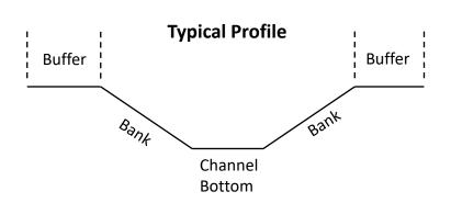
**Note:** This profile represents a typical concrete trapezoidal ditch. Depth, bank slope and buffer area varies.
