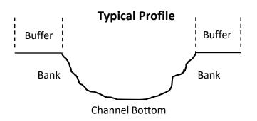
**Note:** This profile represents a typical earthen ditch. Depth, slope and buffer area varies.
