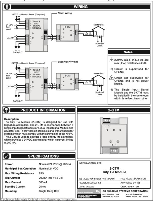
Exhibit A -Signature Loop Controller Installation Sheet for Wiring Specifications
