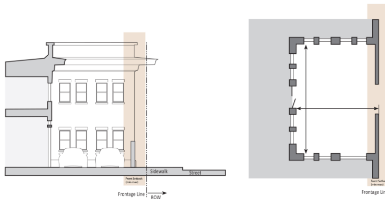
Figure 64-3-6.2 Vehicular Courtyard Frontage Type
