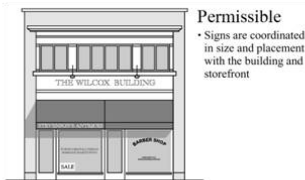
Figure 64-13-7.1 Permissible Signage Placement
